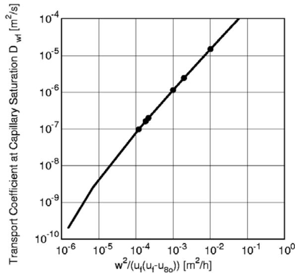
**Fig. 2** Representation of Equation (3) for the graphical determination of  $D_w$ . The values for the materials listed are marked as dots.
